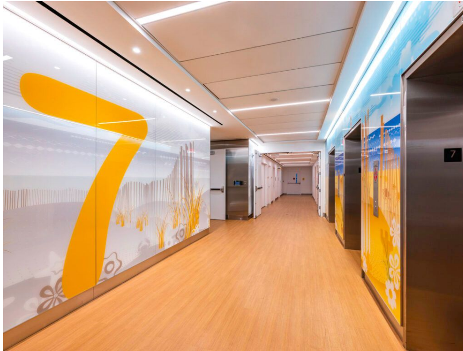
Figure 3: Every corridor requires access to two approved exits, without passing through any intervening rooms or spaces other than corridors or lobbies, per NFPA 101. Courtesy: Geoffrey Lyon, Henderson Engineers
