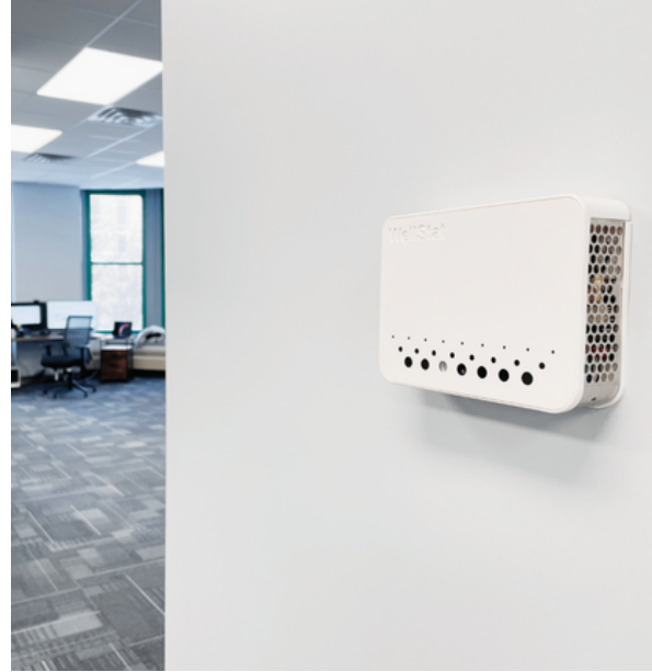
Example of installed WellStat IAQ Wall Mount
