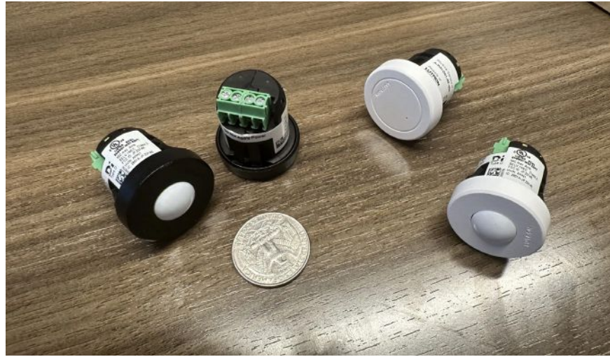
Figure 1: Wireless communication modules and sensors for luminaire level lighting controls are now small enough to allow for mounting in most light fixtures. Courtesy: McGuire Engineers
