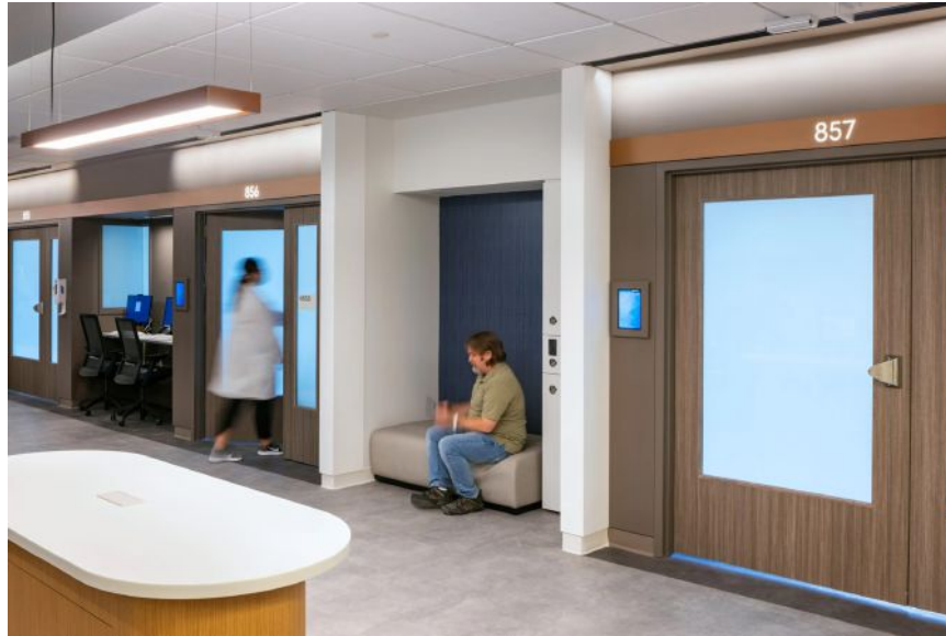
Figure 4: Charting station windows and patient doors on opaque mode for privacy. Courtesy: HDR, Dan Schwalm PennFIRST
