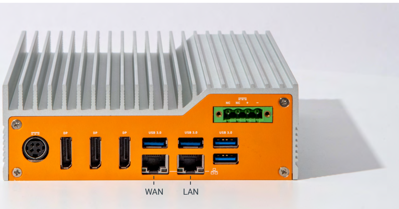
Industrial PCs can deliver dual LAN to alleviate some IT security concerns.
