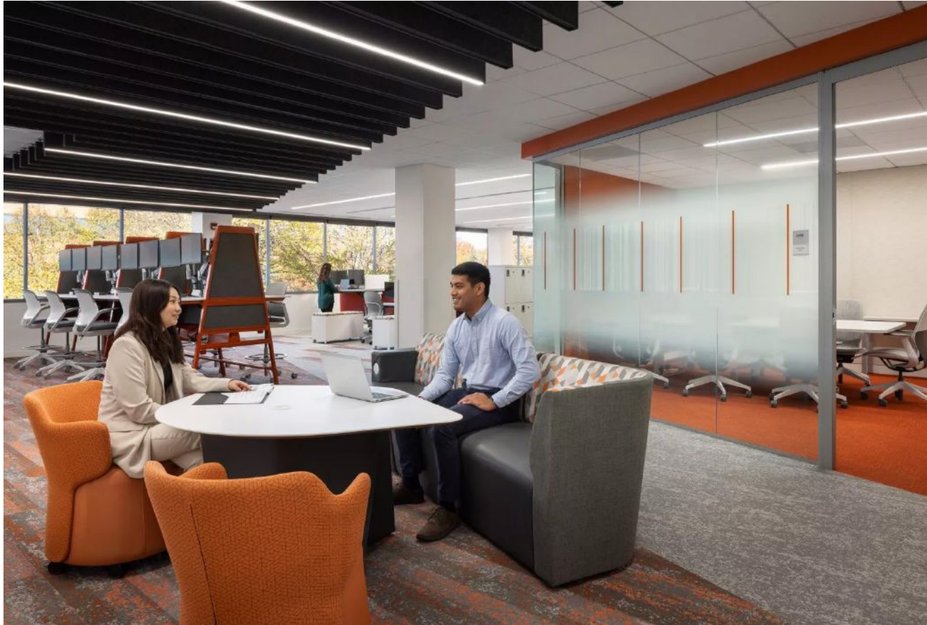
Figure 2: This shows an example of open office lighting that locates the luminaires over the work zone only, leaving the corridor free of unnecessary additional fixtures.
