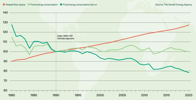
Denmark witnessed a significant reduction in energy consumption for space heating per m<sup>2</sup> in households from the 1990s to the 2020s, thanks to improved insulation, the replacement of oil burners with efficient natural gas boilers and district heating systems, and stricter energy standards for new homes.
