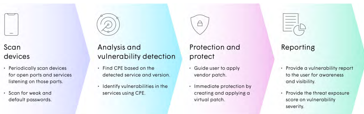
Figure 18—Vulnerability detection and protection solution
