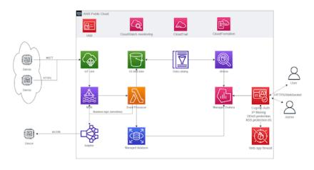
Image 5: DLMS/IEC104 AWS IoT serverless cloud solution
