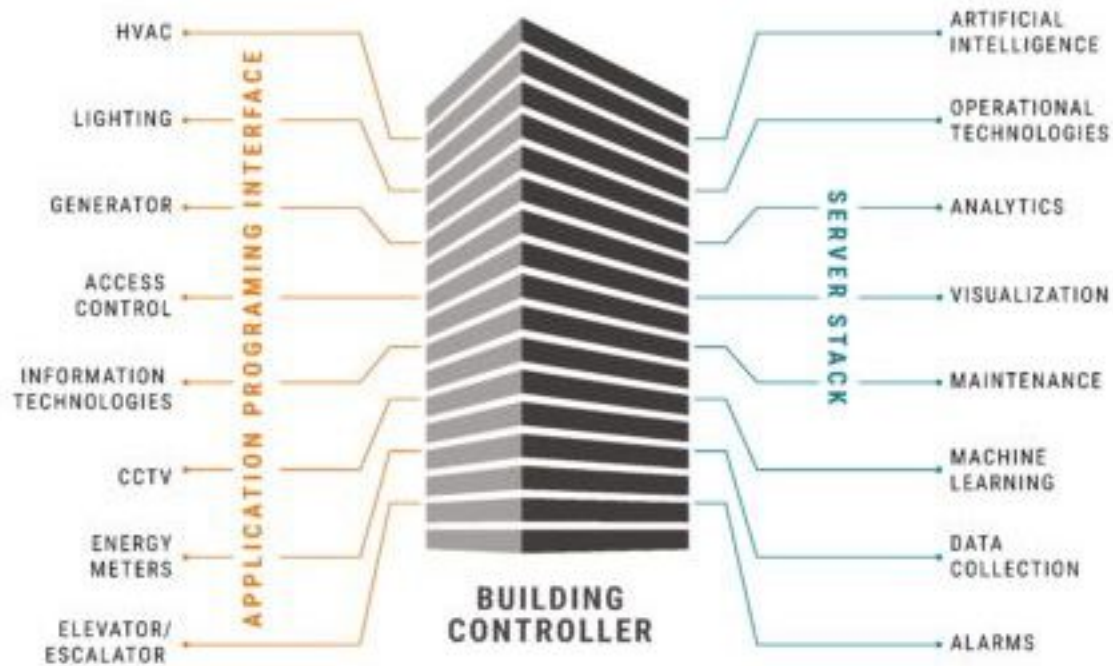
Figure 1: Smart buildings performance is based upon the amalgamation of multiple building systems into a unified building controller to achieve the benefits of remote monitoring and artificial intelligence/operational technology. Courtesy: Stantec
