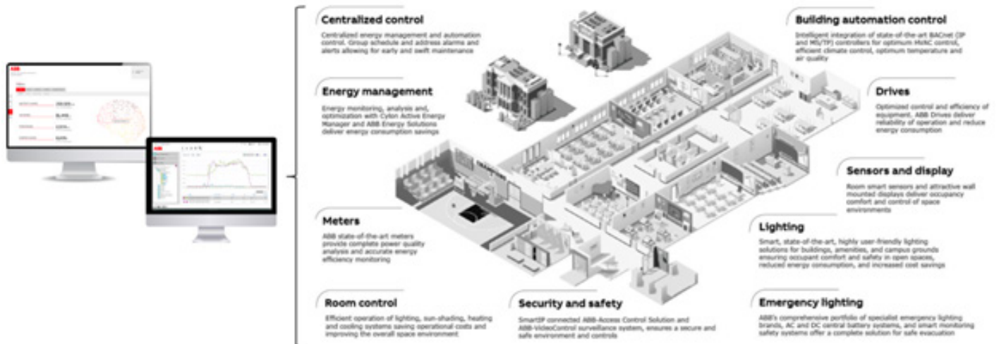
Figure 2: Consolidating facility management systems into a single view
