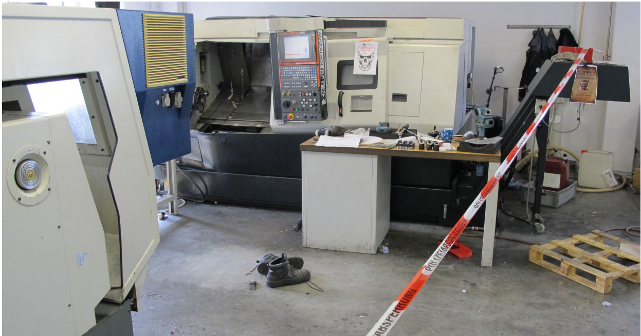
Figure 8-1: Turning machine accident – workpiece knocked out the protective door (source: TÜV SÜD).
