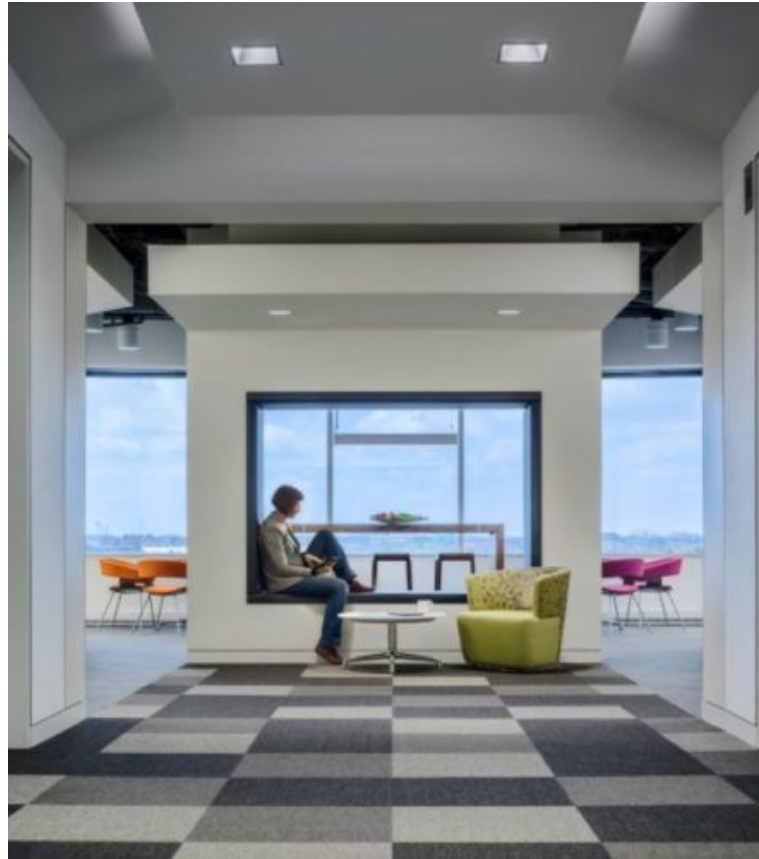
Figure 1: IMEG's architectural lighting design for Zebra Technologies' headquarters features a mix of LED and linear fluorescent lamp sources to minimize energy use and maintenance while remaining cost effective. The control system bridged a variety of protocols and worked in conjunction with the audiovisual system and shading to create one highly functional yet simple-to-use system that will repay the owner in energy savings and an enhanced user experience. Courtesy: Christopher Barrett Photography, IMEG
