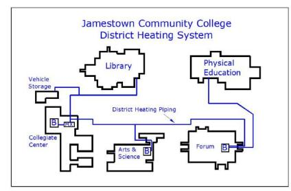
Figure 5: Shown is the district heating system of the Jamestown Community College. Courtesy: Joseph Technology Corp. How solar heat gain affects building design
