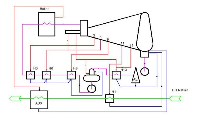
Later the power plant has been repowered with the General Electric LM6000 gas turbine generator designated as unit No. 7. The gas turbine was Figure 1: This shows the initial combined heat and power/district heating system. Courtesy: Joseph Technology Corp.
