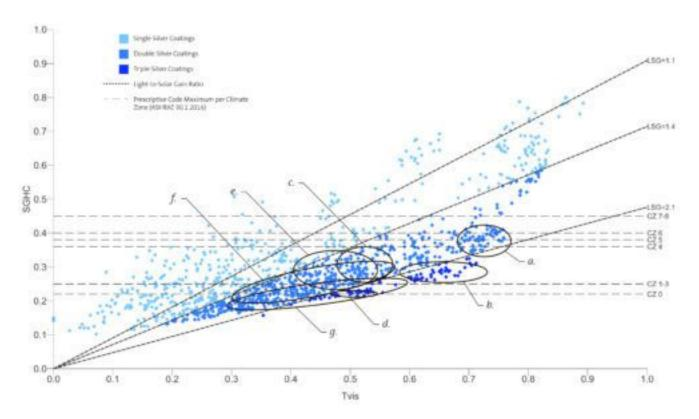
with stringent acoustic requirements particularly for low-end frequencies. While the same solar control coating is applied to each IGU, the center of glass SHGC significantly varies.
