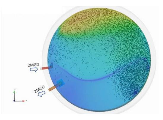
A prime example of this is a CFD study we performed Sin for a client in the central valley region of California, where we used CFD to aid the design of a new pump station intake. Headlosses and flow unevenness were minimized via geometric modifications of the inlet channel an
