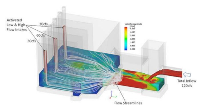
one of the main objectives of the designer is to minimize potential head losses and uneven flow distributions in order to optimize system performance. Asymmetric flows Pump intake operational and geometric optimization using CFD.
