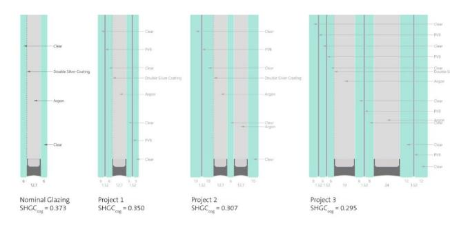
inates, as well as the window unit size and glass-to-frame ratio all additionally modify the total assembly SHGC.
