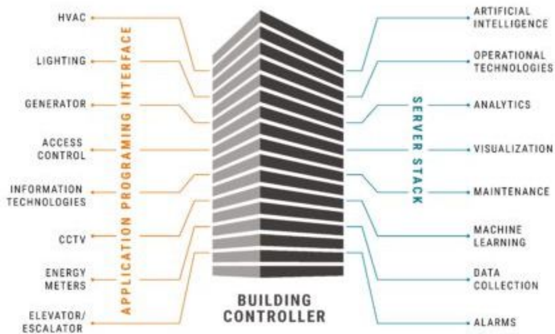
Figure 1: Smart buildings performance is based upon the amalgamation of multiple building systems into a unified building controller to achieve the benefits of remote monitoring and artificial intelligence/operational technology.
