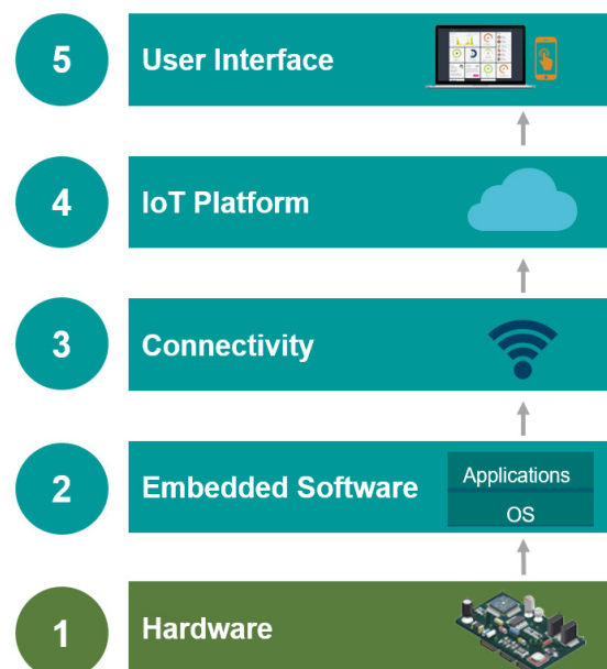
Figure 2: The Enabled IoT Device Stack
