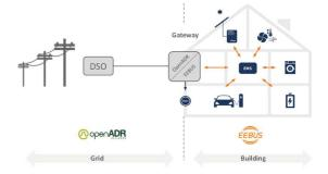
By measuring the power consumption, the DSO may identify hotspots and take in-time corrective action by limiting power consumption via setpoints. In addition to controlling the power demand, the feed-in
