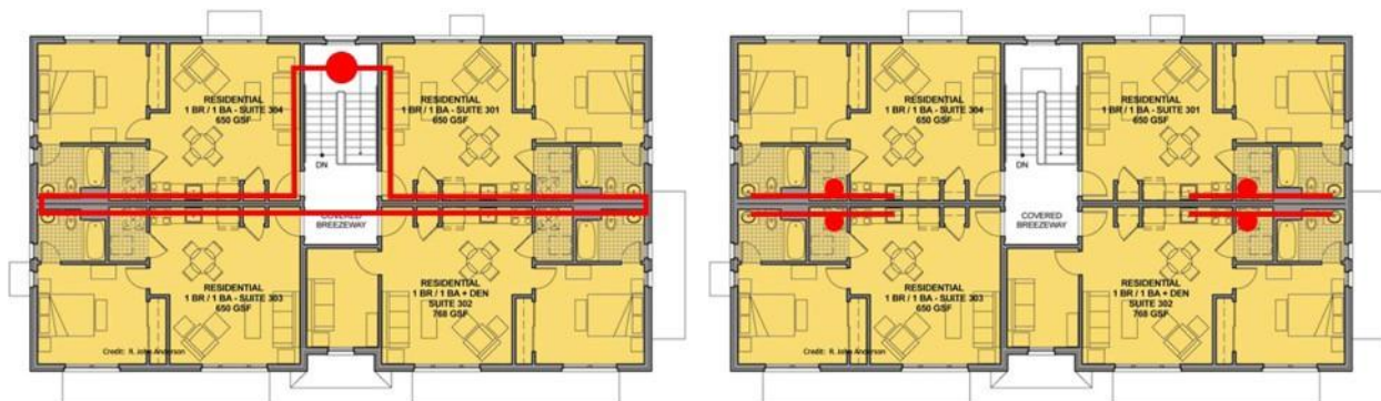
Figure 21. Central Water Heating with Recirculation Loop (left) vs. Individual Water Heaters (right) Connected Directly to the Hot Water Points of Use
