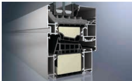
Proposed Window: Passive House certified windows benefit from generous thermal breaks within the frame, typically include triple glazing, and, perhaps most importantly, include gasketing and hardware that ensure airtightness. Photo Credit: Shuco
