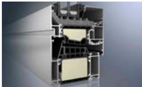
Proposed Window: Passive House certified windows benefit from generous thermal breaks within the frame, typically include triple glazing, and, perhaps most importantly, include gasketing and hardware that ensure airtightness. Photo Credit: Shuco
