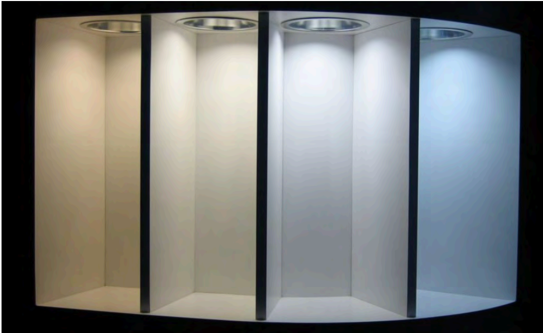
Color temperatures of white light varying 2700K, 3000K, 3500K, and 4100K from left to right. Image courtesy of the Energy and Technology Center, Sacramento Municipal Utility District.
