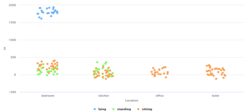
Figure 20. Analysis of the accelerometer data (in the X-direction) for different behavioral patterns associated with different ADLs performed in the given simulated smart home environment.
