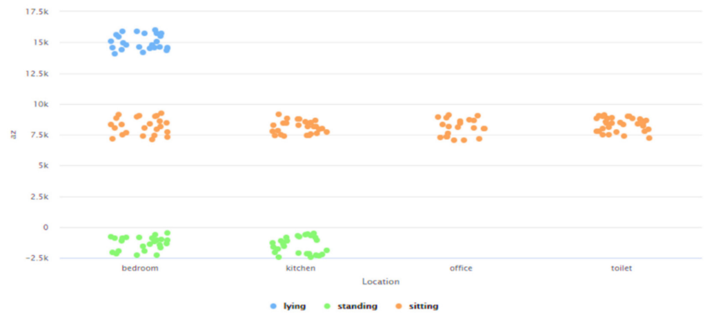
Figure 22. Analysis of the accelerometer data (in the Z-direction) for different behavioral patterns associated with different ADLs performed in the given simulated smart home environment.
