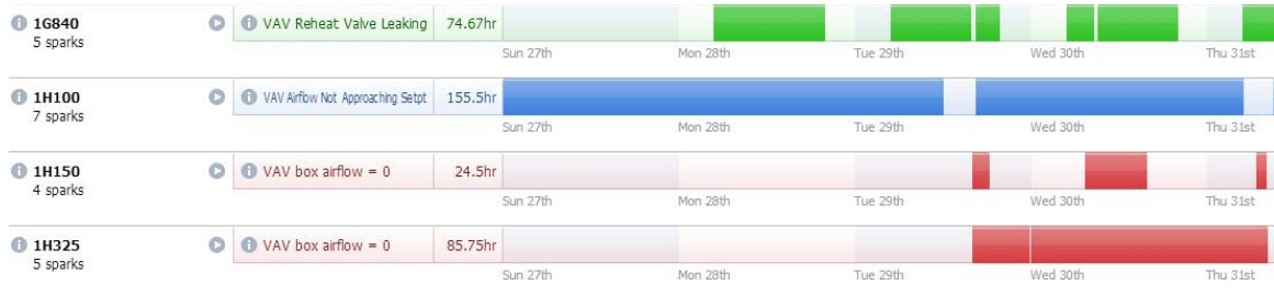
Figure 17. Zone-level fault detection and diagnostics
