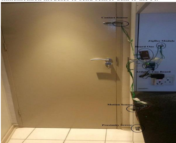
Figure 4.4. Shows Sensors, board and microcontroller deployment at Primary Access Point.
