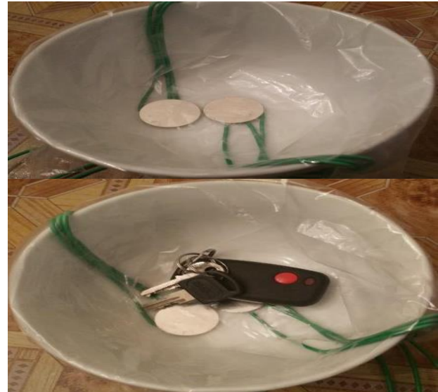
Fig: (a) Shows Piezoelectric sensor deployed in the key bowl. (b) Shows keys placed inside the key bowl.
