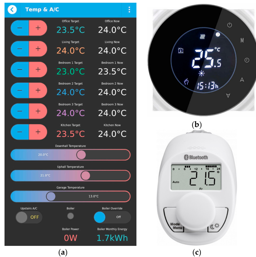
Figure 8. Controlling indoor temperatures with qToggle app (a) together with smart thermostats (b,c).
