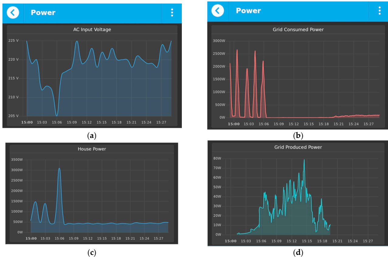
Figure 11. An example of monitoring the power with qToggle: AC Input Voltage (a); House Power (b); Grid Consumed Power (c); Grid Produced Power (d).
