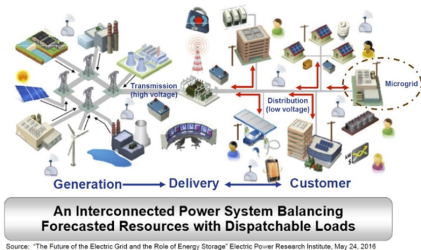
Figure 5.1.10. A “Grid-of-Grids” (EPRI, 2014).
