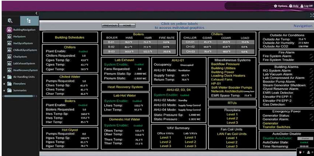
Figure 5: Building automation system control and monitoring software manages a building's various mechanical, electrical and plumbing systems and equipment. Courtesy: SmithGroup
