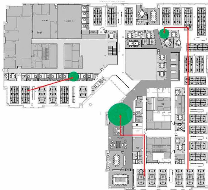
Figure 4: Employees are estimated to save an average of 5 to 15 minutes per week due to the new efficiencies in finding a place to meet and work enabled by the lighting control system working collaboratively to report occupancy status to the native email and room scheduling platform.
