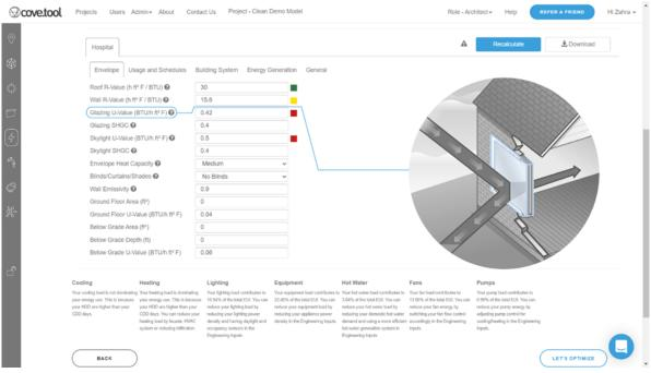
When studying the impact of modifying U-Value on the glazing of the office project, we are able to see that it has a pretty considerable impact. As seen in the graph below, increasing the U-Value from efficient to in-efficient can increase the total building energy use intensity by 105%. For a 53,000 sqft. building this equates to about 40,400\$ in utility bills and 185.4 tons of additional carbon emissions.
