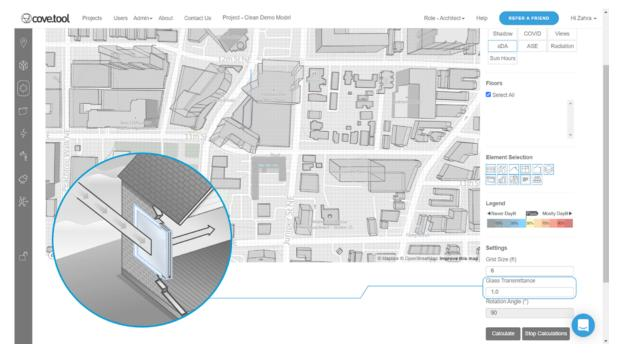
The following graphics demonstrate the Daylight (Spatial Daylight Autonomy sDA) and Glare (Annual Solar Exposure ASE) impact associated with different Visibility Transmittance values for the glazing in the office building. As expected, increasing the visibility transmittance of glass results in admitting more daylight into the spaces which consequently increases the sDA and ASE percentages.
