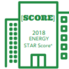
ENERGY STAR score is a normalized 1-100 scale of a building's energy performance against a national dataset of similar buildings, where higher scores signify better energy performance
