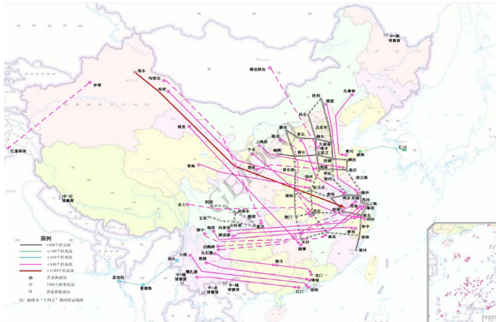
Figure 25: Existing and planned (dashed) UHV lines by 2025 [179] (used with permission)
