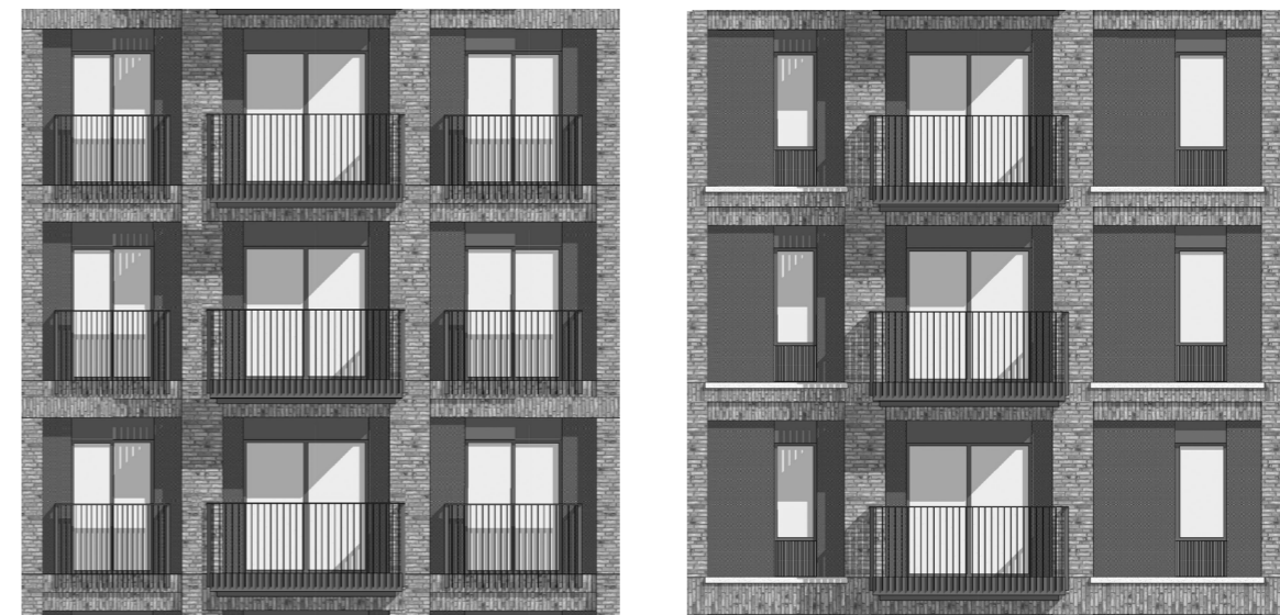
Figure 16: The original design included juliette balconies to most bedrooms (left), however this has been removed for the stretch design to reduce glazing areas (right)
