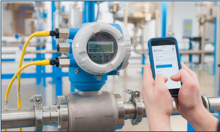
Figure 4: A technician can connect a smartphone to an instrument, such as this Endress+Hauser flowmeter, and access the meter via its integrated web server. The same procedure can also be used for access done from a remote PC or tablet.
