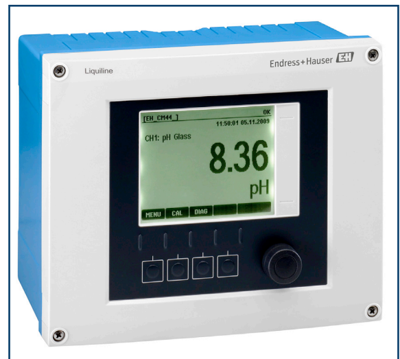
Figure 1: This Endress+Hauser Liquiline transmitter offers EtherNet/IP, Modbus RS485 or TCP, PROFIBUS DP, and HART as well as a web server. This transmitter can communicate with up to eight smart sensors.
