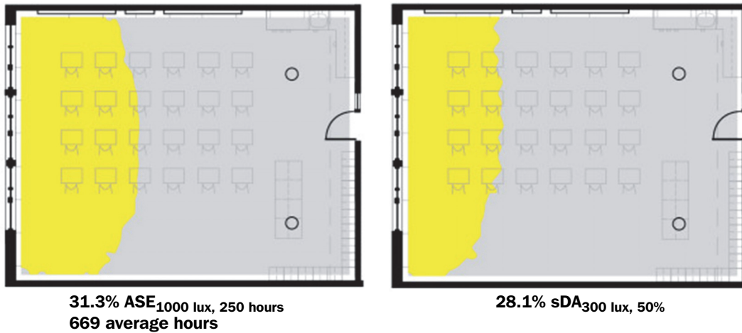
Daylighting illumination levels—initial design.
