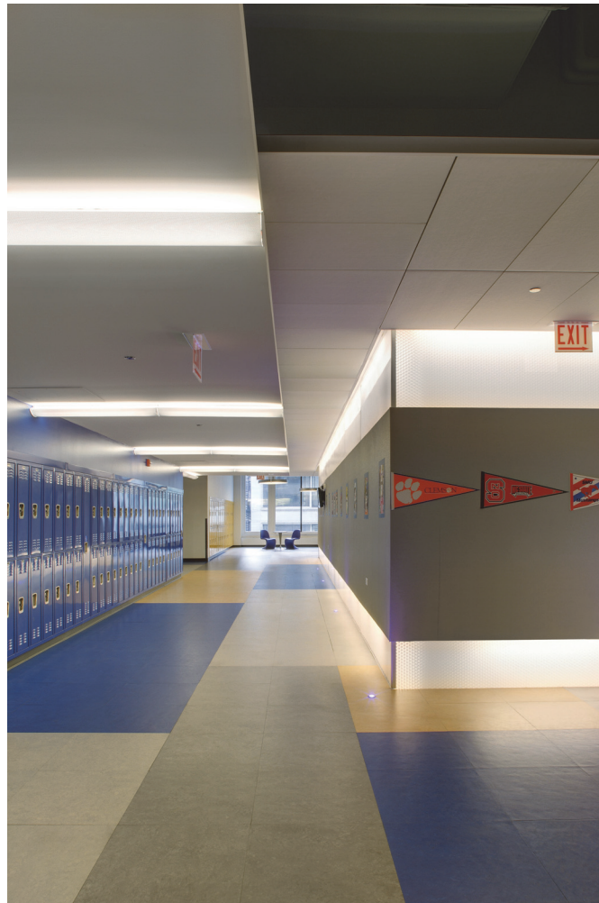
Figure 5-30 (EL10) Lighting as wayfinding.
